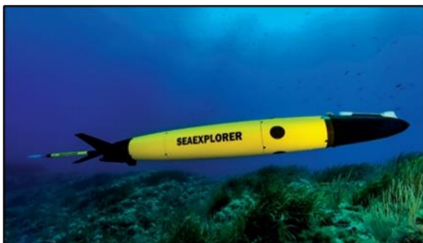
Figure 2 Alseamar Seaexplorer glider
