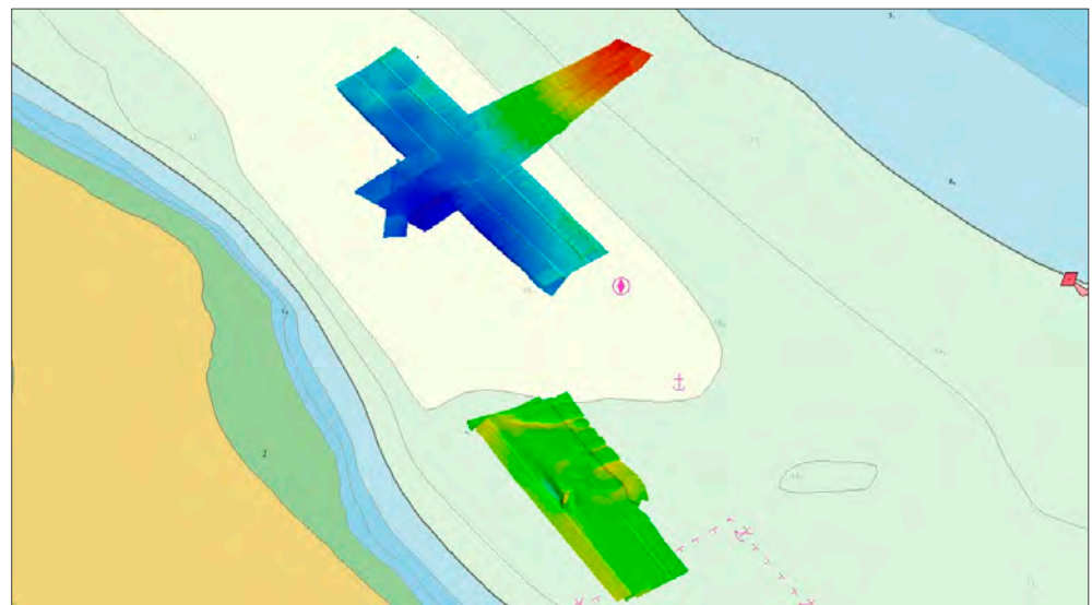
Figure 5. Patch test survey lines for the DriX USV.
